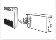
5 The EEV kit has to be installed that the user has no access to it. (built-in type)
